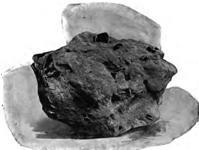
FIG. 65.—Sludge and Old Scale from Boilers Using Water from Scaife Softener.
